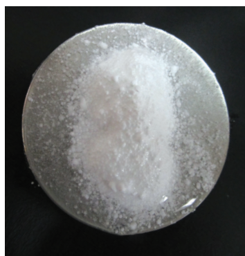
Slotted disk bridged/sealed-off in less than 10 seconds after the application of TriVert™ at a 500 psi differential.
