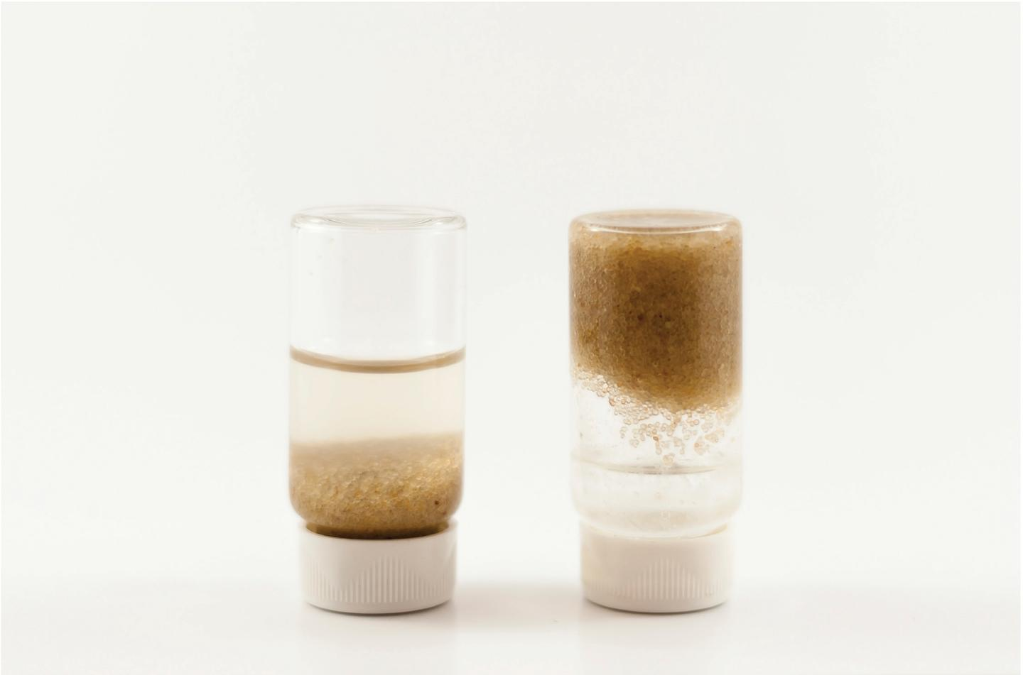
Untreated (left) and SandStill treated sand (right) in slick water
