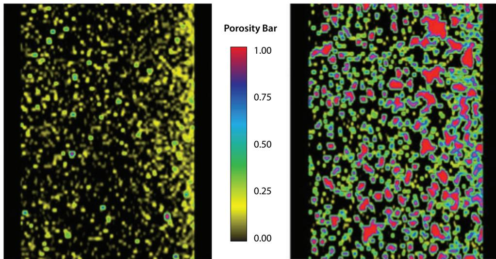
CT scan of untreated (left) and SandStill treated sand (right) in guar/borate system after gel break showing increased porosity
